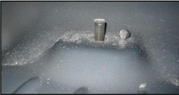
5. ← Cut 1/2" of length off the threaded stud protruded from the floor where the metal bracket was attached to. This stud is too long for the lower panel to fit properly, and must be cut. By only cutting 1/2" off, the stud is still reusable for mounting your seats back into the car at a later time if desired.
