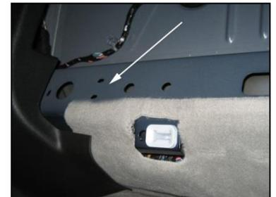
**Optional:** The metal hook/latch in the Camaro at the top of the rear panel is not removable; therefore this will protrude through the Rear Seat Delete. If your car is not Black, we recommend using a black paint marker or Sharpie to color this metal hook so that it blends into the new panel properly, for a clean look.
