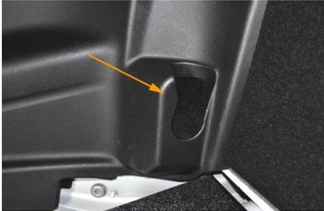
2. ← Use a 5" x 5" piece of black carpet from your hardware kit to cover the area where the seat back pins were located.
