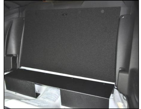
4. Install the Back Panel into the car and insert the 4 supplied plastic pushpins into the top area that aligns with the 4 holes in the upper shelf. →
