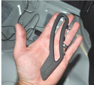
5. ← Carefully pry the small plastic side panel insert labeled with "airbag" out of the main side panel around the seat belt strap. You will need to slide this off of the seatbelt strap.
