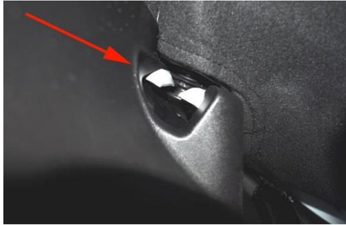
3. ← Remove Back seat assembly: Fold seat backs down. On each side is a metal spring-loaded clip holding the seat pin in place (see photo). Yank upwards on that pin to dislodge it. If its stuck, you may need to pry the spring loaded washer towards the center of the car while yanking upwards. Once the pin comes loose, lift that seat back up at a 45 degree angle and pull it towards the outside of the car to slide the inner pin out of it's hole. Remove the seat back from the car.
