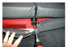
• ← Remove the black Torx head screws (**T40**) holding the rear seat structure in place.
