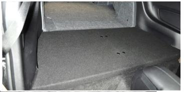
3. • Install the lower panels in the car. Push the 4 smaller "shiny" push pins through each of the lower panels in the pre-drilled holes, into the flat support brace underneath. (2 extra pins are included in case of breakage) NOTE: For best results, you may have to use one hand under the panel to lift up the support brace as you push the pin through from the top, to get the pin completely flush.
