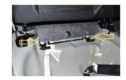
10. ← On the driver side under the side panel, is a wiring harness with a black clip attached to a post. Remove this plastic clip from the post and let the wire hang down.
