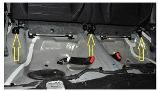
3. ← Fold the seat backs down. There is one more nut to remove at each side near the side panels. Remove the seat backs from the car.
