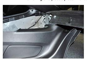
5. ← Remove the rear side panels by firmly pulling away from the body of the car to release the plastic clips holding it in place. This may take more force than you think is comfortable, but just pull firmly around the edges and each one will release.
