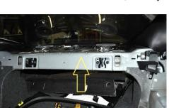
12. ← With the side panels gone, you can temporarily remove the factory carpeted rear deck panel. This will be reinstalled in a later step.
