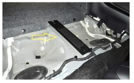
1. • Install the flat center brace over the transmission tunnel using the two fat plastic push pins included in the hardware kit. One push pin goes in the
