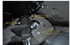
Remove the two bolts holding each of the two black metal brackets used for the child seat mounting points. Plug the holes by reinstalling the bolts here.
