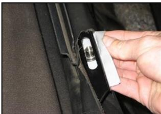
3. ←The threaded T-nuts must be set in place **BEFORE** you install the Rear Seat Delete back section. Use a piece of duct tape to firmly hold each T-nut centered in the 2 slots shown in the photo. (You will be screwing the supplied bolts through the RSD and into this T-nut.)
